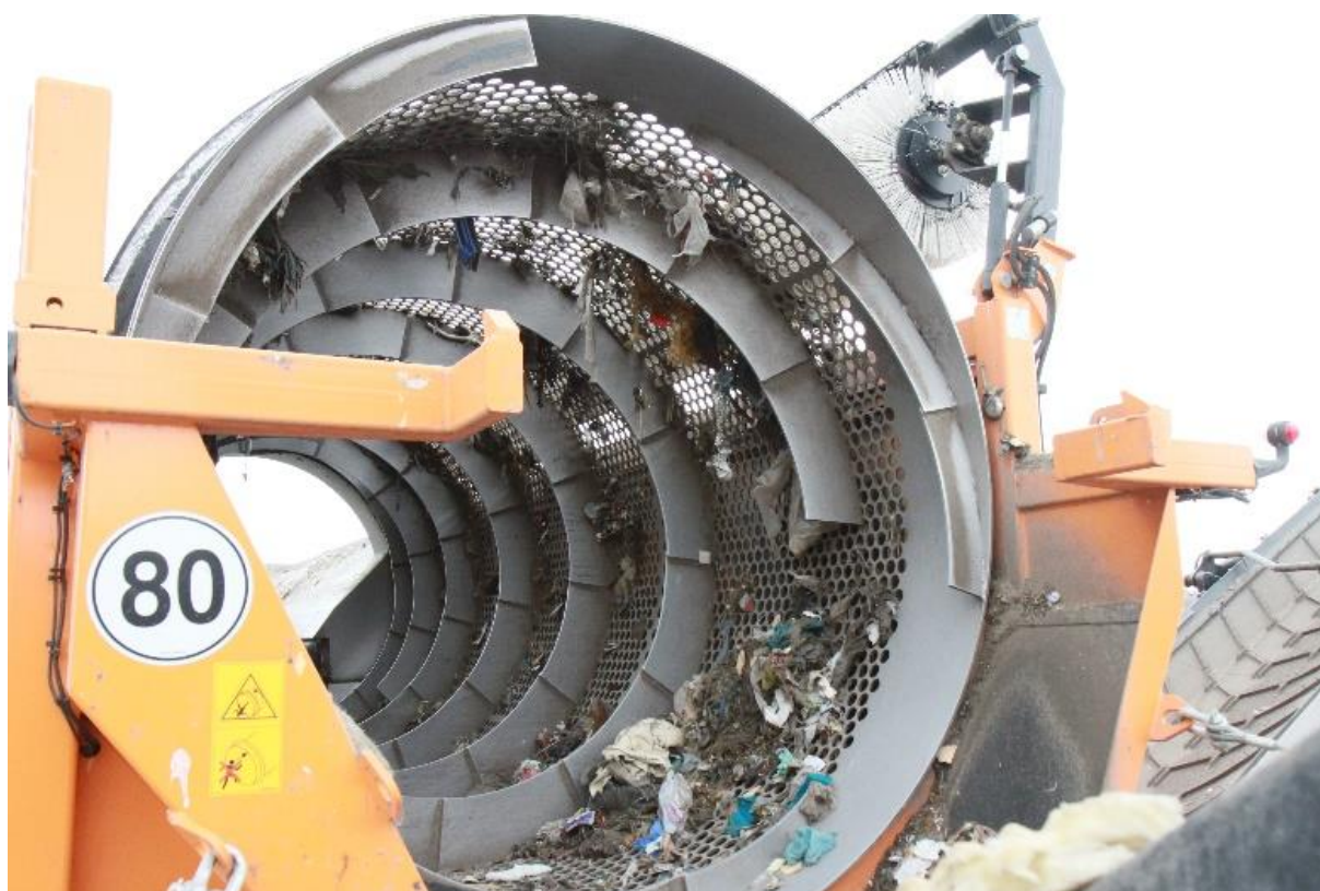
Figure 5 - Mechanical pre-treatment operation (rotary sieve) at the Zdechovice landfill in the Czech Republic
