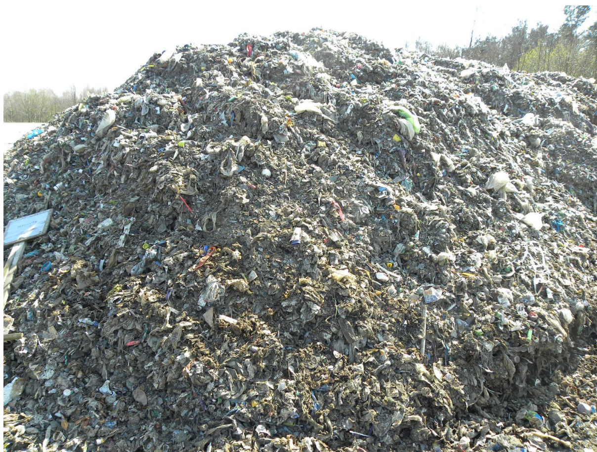
Figure 13 - Waste after stabilisation in composting cells at the Janczyce landfill in Poland
