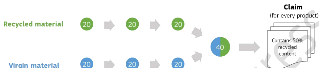
Figure 5. Exemplary scheme of the controlled blending model
