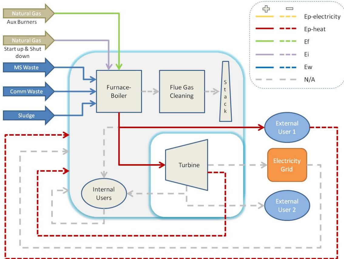
Note: The graphic representation is not entirely correct as Ep-heat takes into account the total amount of steam exit boiler (i.e. to turbine and to external user 1) and the temperature and pressure entering the steam condensate system (i.e. 45 °C and 5 bara) also for the total steam flow.
