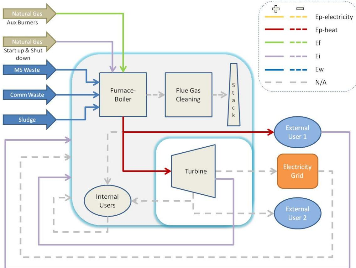
Note: The graphic representation is again not entirely correct as the total amount of steam exit boiler (i.e. to turbine and to external user 1) is used for Ep-heat and the temperature and pressure entering the steam condensate system (i.e. 45 °C and 5 bara) also for the total steam flow are used in Ei.
