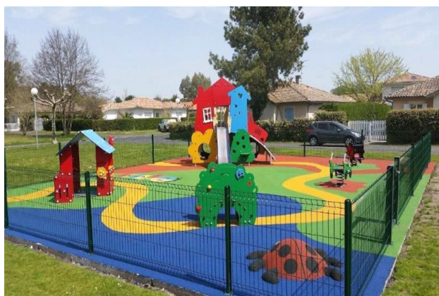
Figure 2. Example of a recreational playground made using SBR from ELT as a base layer (i.e., under the coloured EPDM layer).
